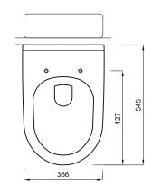
**Special notes** Pan fixes to floor using side fixing bracket supplied with pan.
